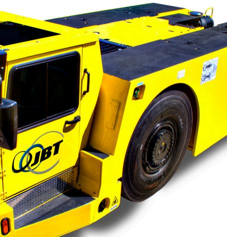
4 wheel steer with 3 positions, reduces turning radius to improve maneuverability in cramped operating conditions
