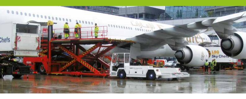
The CARGO MASTER TRANSPORTER CMT 7 is specifically designed for transport of heavy and sensitive airfreight. As a link between Cargo Loader and Dolly Train, these transporters notably increase the clearance capacity on large international airports.
