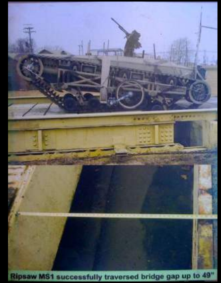
Ripsaw MS1 successfully traversed bridge gap up to 49"
