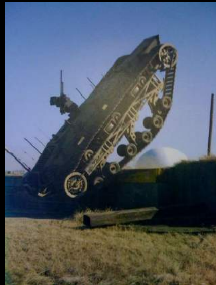
Ripsaw MS1 successfully climbed 60% Grade Slope
